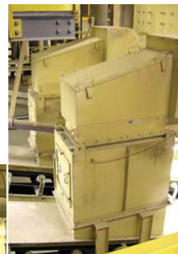
Dalamatric insertable collectors (the tops are slanted) are venting each raw material silo in this room at the top of a batch house. Clean-side access for service eliminates the need for OSHA “confined space” entry permits and procedures.
